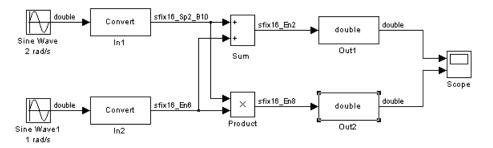
In the model, the data type displayed with the In1 block indicates that the output data type name is sfix16\_Sp2\_B10. This corresponds to fixdt(1, 16, 0.2, 10) which is a signed 16 bit fixed-point number with slope 0.2 and bias 10.0. The data type displayed with the In2 block indicates that the output data type name is sfix16\_En6. This corresponds to fixdt(1, 16, 6) which is a signed 16 bit fixed-point number with fraction length of 6.
