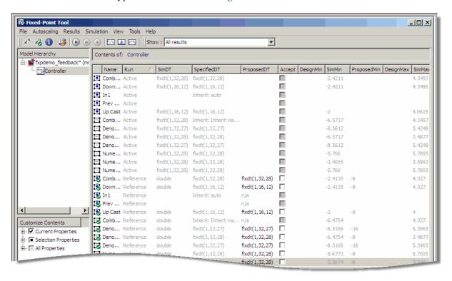
7 In the Model Hierarchy pane of the Fixed-Point Tool, select the fxpdemo feedback system. In the Contents pane, select the Transfer For block named Analog Plant that corresponds with either the active or the reference run, and then click the **Time Series Difference (A-R) Plot** button .
