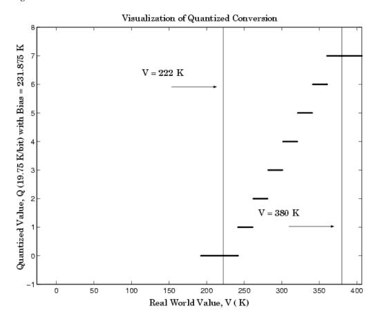
The quantization error is -9.875 K/bit  $\leq Error \leq 9.875$  K/bit, which is approximately 2.5 times smaller than the error associated with the purely linear conversion.
