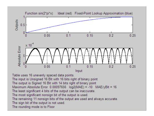
The upper plot shows the ideal function  $\sin(2\pi x)$  and the fixed-point lookup approximation between the breakpoints. In this example, the ideal function and the approximation are so close together that the two graphs appear to coincide. The lower plot displays the errors.
