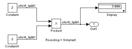
Because the simulation uses multiplication followed by shifts to handle the net slope correction, net slope precision loss occurs. This precision loss results in numerical inaccuracy: the calculated product is 3.999, not 4, as you expect.
