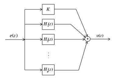
As in the series canonical form, there is no unique description for the first-order and second-order transfer function. Because of the nature of the Sum block, the ordering of the individual filters doesn't matter. However, because of the constant K, you can choose the first-order and second-order transfer functions such that their forms are simpler than those for the series cascade form described in the preceding section. This is done by expanding H(z) as
