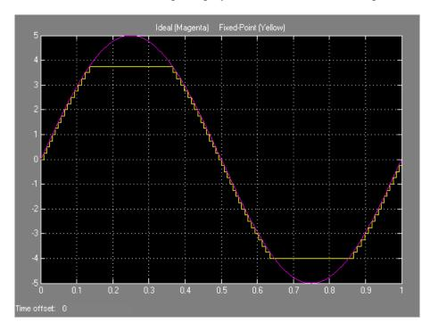
The simulation demonstrates the quantization effects of fixed-point arithmetic. Using a 5-bit word with a precision of  $(1/2)^2 = 0.25$  produces a discretized output that does not span the full range of the input signal.
