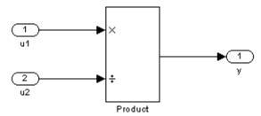
As discussed in "Fixed-Point Numbers" on page 2-3, each fixed-point quantity is calculated using its slope, bias, and stored integer. So in this example, not only is there the high-level divide called for by the block operation, but intermediate additions and multiplies are performed:
