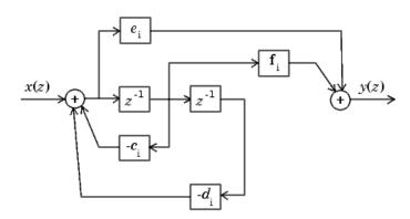
$$\frac{y(z)}{x(z)} = \frac{e_i + f_i z^{-1}}{1 + c_i z^{-1} + d_i z^{-2}}$$
