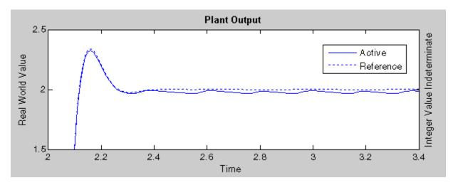
The plant output signal represented by the active run achieves a steady state, but a small limit cycle is present because of poor A/D design.
