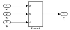
As stated in the C standard, the most efficient rounding mode for multiplication operations is always floor. However, the C standard does not specify the rounding mode for division in cases where at least one of the operands is negative. Therefore, the most efficient rounding mode for a divide operation with signed data types can be floor or zero, depending on your production target.
