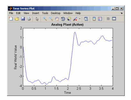
The preceding plot of the plant output signal reflects the initial guess at scaling. The Bode plot design sought to produce a well-behaved linear response for the closed-loop system. Clearly, the response is nonlinear. Significant quantization effects cause the nonlinear features. An important part of fixed-point design is finding a scaling that reduces quantization effects to acceptable levels.
