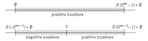
For both the signed and unsigned fixed-point numbers of any data type, the number of different bit patterns is  $2^{ws}$ .
