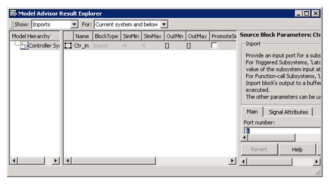
The Model Advisor Result Explorer opens, displaying the Inport blocks that do not have an output minimum and maximum specified.
