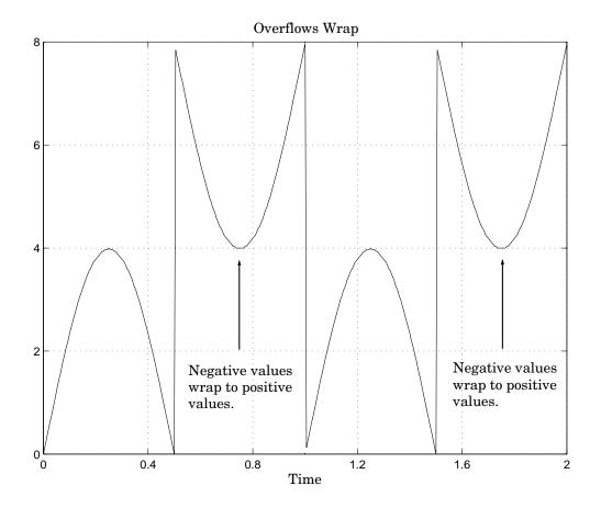
**Note** For most control applications, saturation is the safer way of dealing with fixed-point overflow. However, some processor architectures allow automatic saturation by hardware. If hardware saturation is not available, then extra software is required, resulting in larger, slower programs. This cost is justified in some designs—perhaps for safety reasons. Other designs accept wrapping to obtain the smallest, fastest software.
