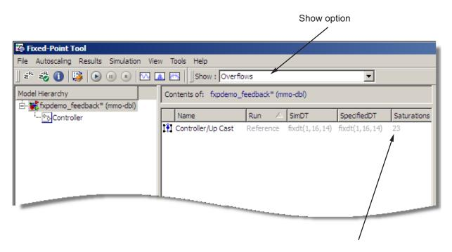
Number of Saturations for Controller/Up Cast block
