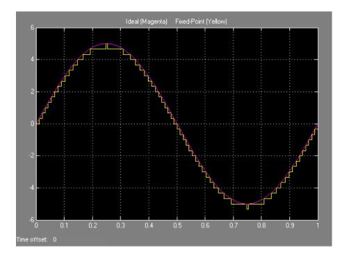
You do not need to find the slope using this method. You need only the range of the data you are simulating and the size of the fixed-point word used in the simulation. You can achieve reasonable simulation results by selecting your scaling based on the formula
